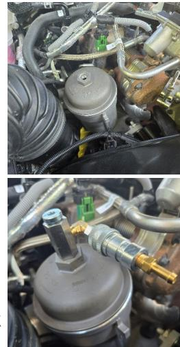
3. Your kit includes a replacement aluminum oil fill cap with a port already in it (FPFC-CUM). Replace OE cap with Frantz cap, but do not throw away OE cap (save this in case you remove filter system from vehicle).
